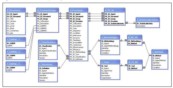
Figure 2 - Structure of the repository
